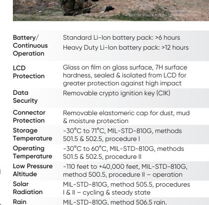
procedure I - rain & blowing rain
